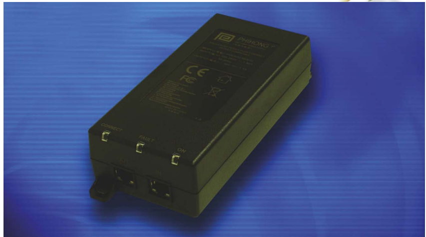
Figure 2 Legacy Ethernet systems can include POE capability with the addition of a midspan power supply that injects a POE voltage into the network. The single-port POE 60U-560G from Phihong provides 60W and costs $62 (one).
